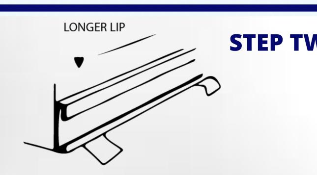
Make sure the longer lip of the C-section is uppermost & line up its lower edge with the bottom of the fascia, ensuring it is horizontal so that the curtain hangs smoothly. Press each end lightly so you can make any adjustments.
