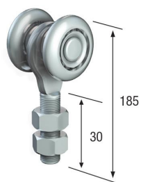
SLIDE-10-WH-30 Galvanised steel 2 Wheel hanger with short 30mm thread
