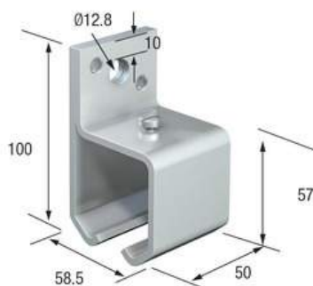
SLIDE-10-WB-F Galvanised steel Single wall bracket - face fix
